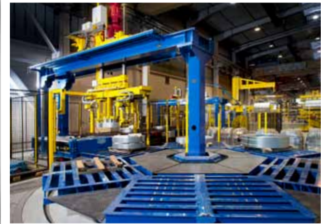
Coil stacking with mandrel clamping in the coil eye and outside gripper
